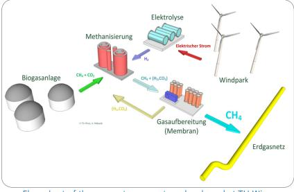
Flow chart of the power-to-gas system developed at TU Wien
