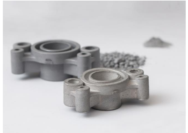
Aluminium alloy MIM component (background: injection moulding part, feedstock, powder)
