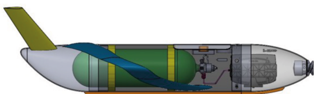
Schematic of component arrangement in UAS fuselage
