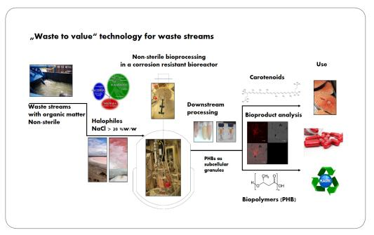
Transformation of >95% organic content of waste streams into valuable products, like carotenoids or biopolymers – e.g. for use in food- and pharmaceutical industry or packaging and plastics indusry
